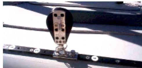
**Figure 32** *Jib block with standup spring in place*
