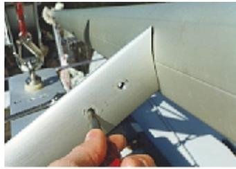
**Figure 3** Lining up holes on spreader
