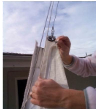
**Figure 33** *Jib head and zipper luff detail*
