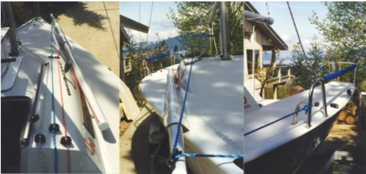
Figure 39 Spinnaker line details: halyard (next to companionway), tack line (blue) and bowsprit (red)
