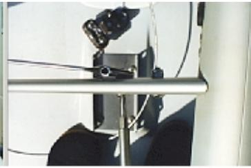
**Figure 4** Tightening spreader bolts
