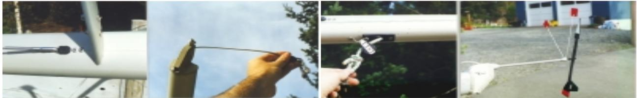
**Figure 10** Lower shroud in place      **Figure 11** Main and spinnaker halyards being pulled out of the mast      **Figure 12** Windex attached to top of mast
